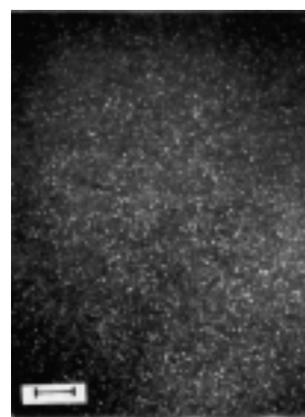
Figure 1. The transmission electron micrograph of \text{TiO}_2 nanoparticles record on JEOL 2000-EX with working voltage 120 kV (dark field). Scale is 200 nm.
